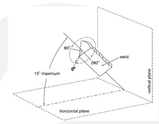
The longitudinal axis of the weld may be inclined no more than 15° with respect to the horizontal plan. The centre of the weld face "C" must lie within the rotational limits of 80° to 280° as shown.
