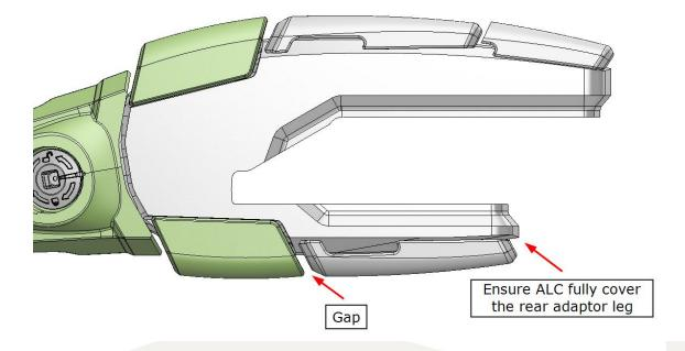
Final position how ALC are placed over the Adaptor is as below.
