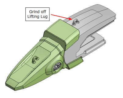
Two ALC can be used to fit over the top leg of the Adaptors by fully utilizing one uncut and the other partially cut to fill up the remaining leg length. Position the ALC on the top leg of Adaptor. Ensure the gap between HD Wear Cap and ALC is not more than 10mm.
