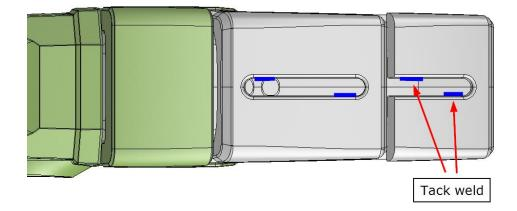
Preheat the Adaptor and ALC area to be welded to 150°C before proceeding with complete weld. Start welding on the area around the wear cap as specified in the figure below with a weld size of 20mm to 25mm fillet as shown. Mechanical attached GET should be removed prior the preheat and welding of the ALC.
