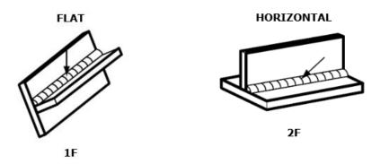
Deviation from the Flat or Horizontal position is permissible as shown in figure below as typically described in welding standard AWSD1.1, Structural Welding--Steel, Figure 4.2 "Positions of Fillet Welds".
