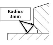
Weld Before Grinding
